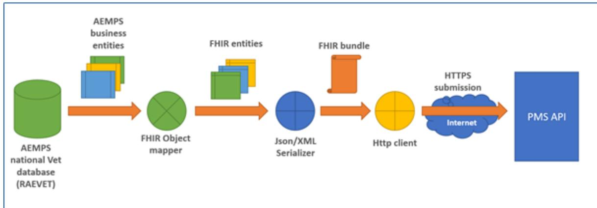
Figure 5: Client architecture for testing the API SPOR V2
